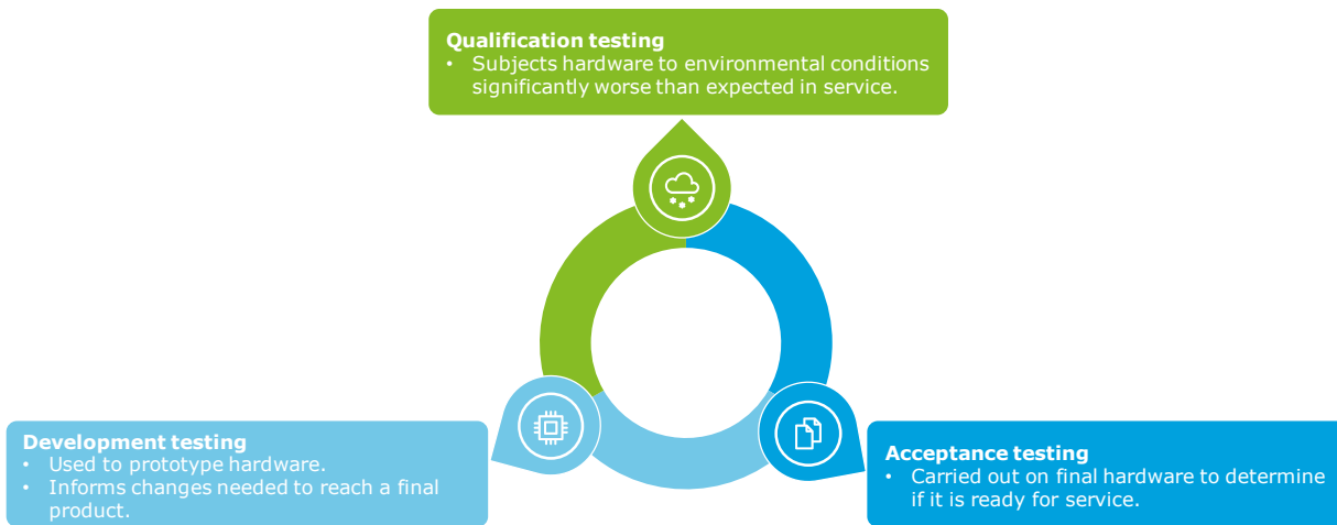
Figure 4.1 Aerospace hardware testing stages
